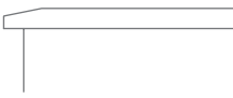
Top with Large Bevel SST-LB Adds ¾" to overall height. Adds 1½" to overall width. Adds ¾" to overall depth.
