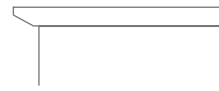
Top with Reverse Bevel SST-RB Adds ¾" to overall height. Adds 2" to overall width. Adds 1" to overall depth.
