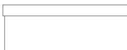
Top with \frac{1}{8} " Overhang EST-MO Adds \frac{3}{4} " to overall height. Adds \frac{1}{4} " to overall width. Adds \frac{1}{8} " to overall depth.
