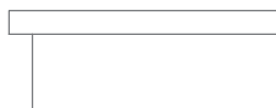
Top with \frac{3}{4} " Overhang EST-TR Adds \frac{3}{4} " to overall height. Adds 1½" to overall width. Adds \frac{3}{4} " to overall depth.
