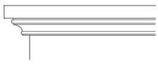
Top with Trim SST-CH Adds ¾" to overall height. Adds 2" to overall width. Adds 1" to overall depth.
