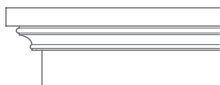
Top with Trim SMT-CH Adds 1" to overall height. Adds 2" to overall width. Adds 1" to overall depth.
