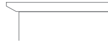
Top with Reverse Bevel SBT-RB Adds 1" to overall height. Adds 2" to overall width.
