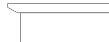
Top with Reverse Bevel SMT-RB Adds 1" to overall height. Adds 2" to overall width. Adds 1" to overall depth.
