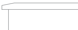
Top with Large Bevel EST-LB Adds \frac{3}{4} " to overall height. Adds 1½" to overall width. Adds \frac{3}{4} " to overall depth.
