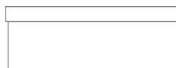
Top with 1/8" Overhang SST-MO Adds ¾" to overall height. Adds ¼" to overall width. Adds 1/8" to overall depth.
