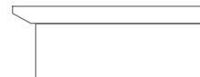
Top with Reverse Bevel EST-RB Adds \frac{3}{4} " to overall height. Adds 2" to overall width. Adds 1" to overall depth.
