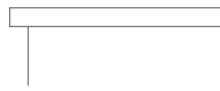
Top with ¾" Overhang SST-TR Adds ¾" to overall height. Adds 1½" to overall width. Adds ¾" to overall depth.
