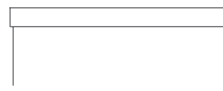
Top with 1/8" Overhang SST-MO Adds ¾" to overall height. Adds ¼" to overall width. Adds 1/8" to overall depth.
