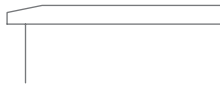
Top with Large Bevel SBT-LB Adds 1" to overall height. Adds 1½" to overall width.
