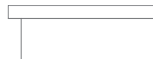
Top with \frac{3}{4} " Overhang SMT-TR Adds 1" to overall height. Adds 1 \frac{1}{2} " to overall width. Adds \frac{3}{4} " to overall depth.
