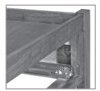
**STEP 5:** Extend the drawer slides. Place the drawers onto the slides and slide them into place. The slides should catch when the drawer is fully closed.
