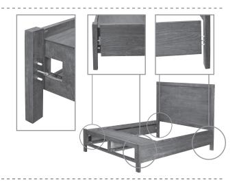
**STEP 4:** Slide the curved washer in place (as shown) and tighten the nut with the wrench provided.
